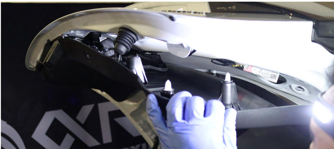
If your Tesla Model 3 is equipped with a power liftgate trunk, ensure to unplug the wire while removing the trunk panel.
