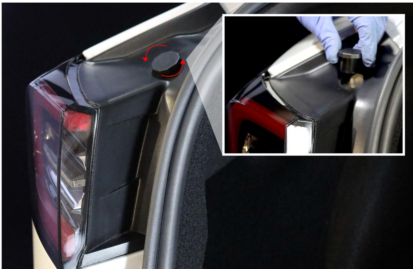
Open the side of the carpet and proceed to remove the two 8mm nuts from the back of the tail light.
