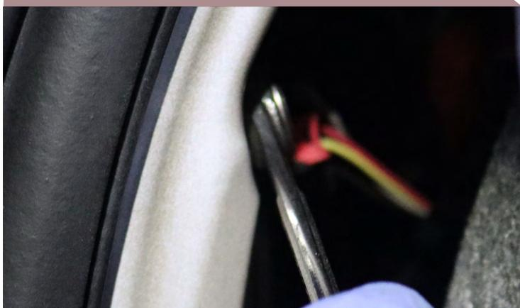
Disconnect the tail light wires.
