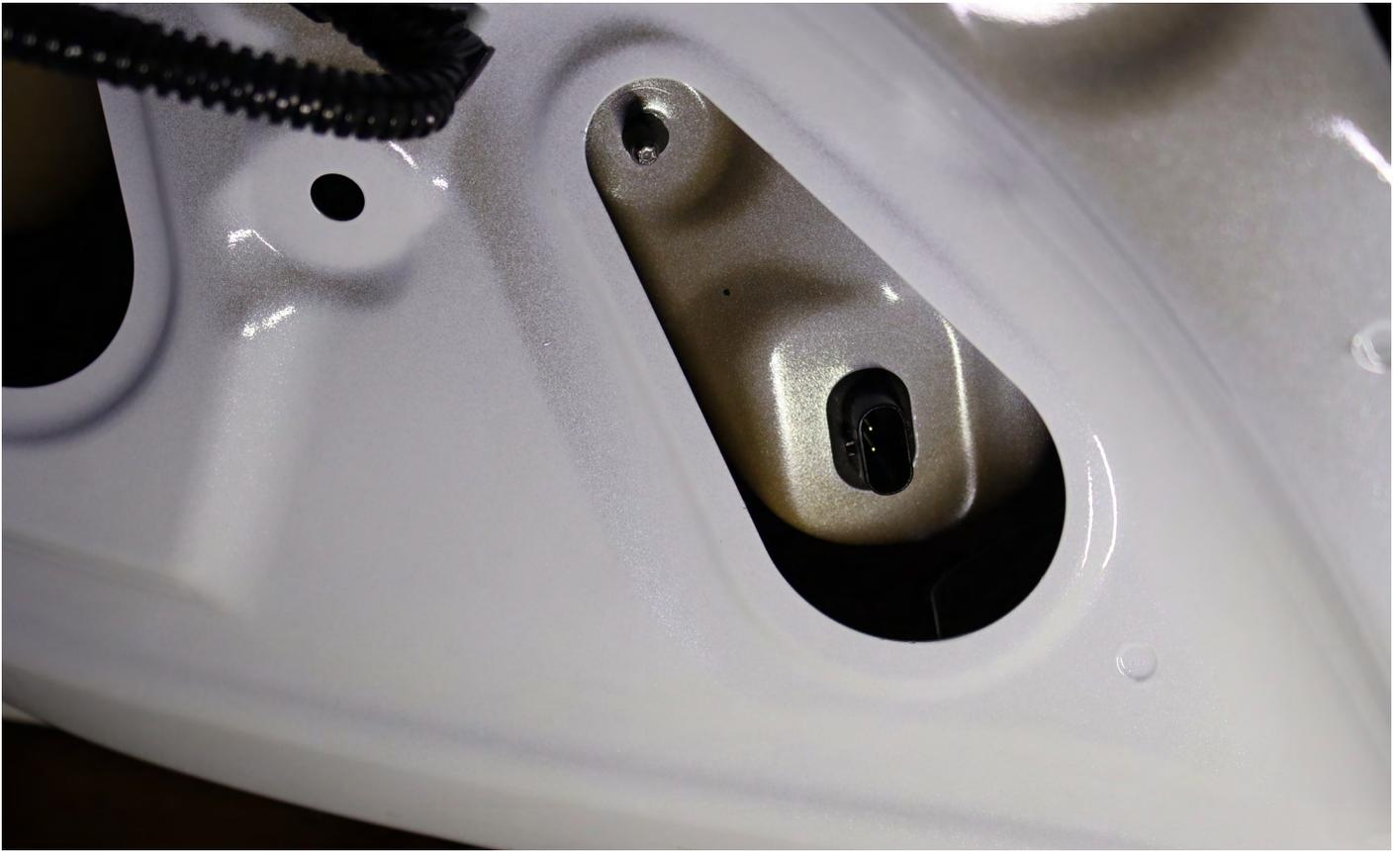
Using a plastic plier, delicately pull and detach the inner section of the tail lights.
