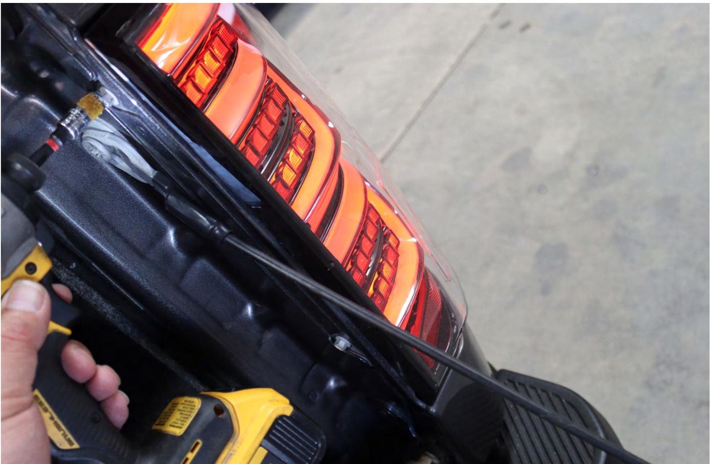
Tighten the 2 X 8mm bolts for each side. NOTE: When using a power wrench, ensure not to overtighten the bolts.
